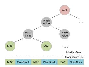
Fig. 10. The build process of Merkle-Tree
