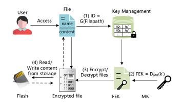
Fig. 5. The access to file process of VACUUM
