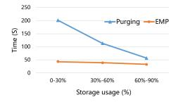
Fig. 15. The time overhead of different memory usages under Purging and EMP when deleting files with the same size
