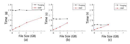
Fig. 14. The time overhead of Purging and EMP to delete different file sizes
