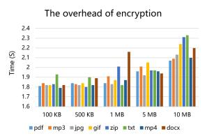
Fig. 11. The encryption overhead
