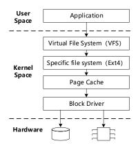
Fig. 2. The process of data storage
