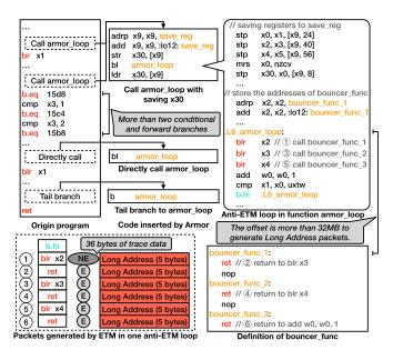
Fig. 5. The details of loop functions.
