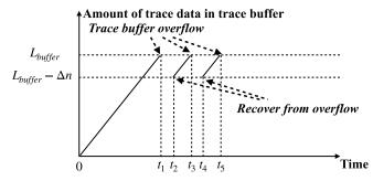
Fig. 2. The model of trace buffer overflow.
