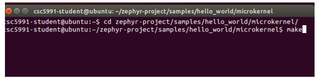
The above screenshot of make will build the hello\_world sample application using the default settings defined in the application's Makefile. You can build for a different platform by defining the variable BOARD with one of the supported platforms, for example:
