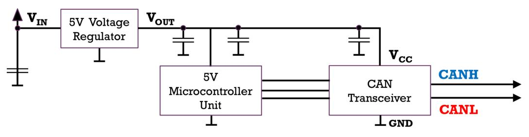
A typical connection of ECU to CAN
