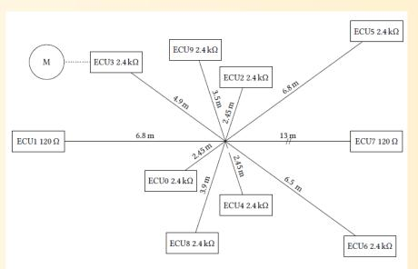
CAN topology of the prototype setup
