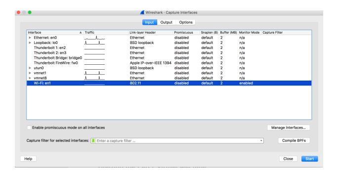
The screenshot below shows the configuration of the capture interface in Wireshark program on my iMac with promiscuous. You need to enable promiscuous mode and configure the Link-layer Head as Per-Packet Information.
