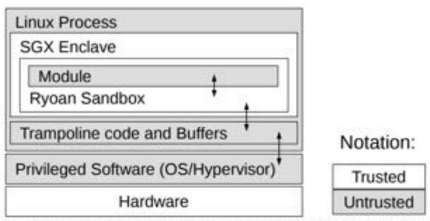
Figure 1: A single instance of Ryoan's distributed sandbox. The privileged software includes an operating system and an optional hypervisor.
