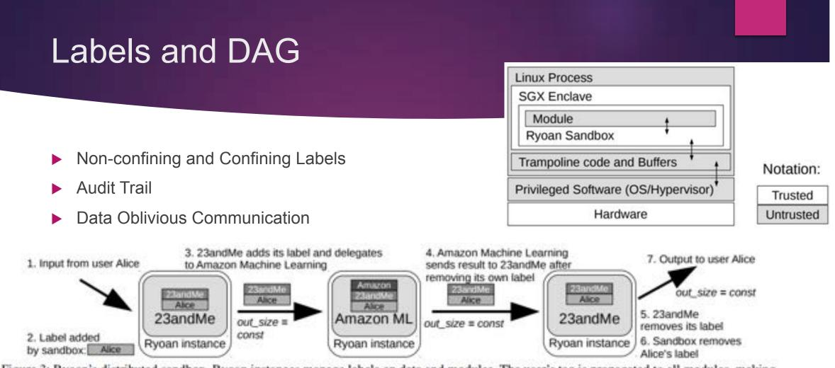
Figure 3: Ryoan's distributed sandbox. Ryoan instances manage labels on data and modules. The user's tag is propagated to all modules, making them confined after receiving input; For example, 23andMe's tag is kept when it outsources to Amazon Machine Learning to prevent leaking secrets from 23andMe.
