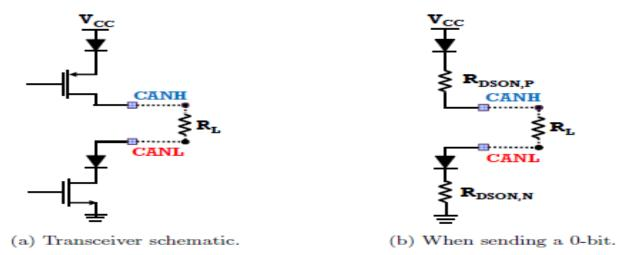
Figure 2: Output schematics of a CAN transceiver.
