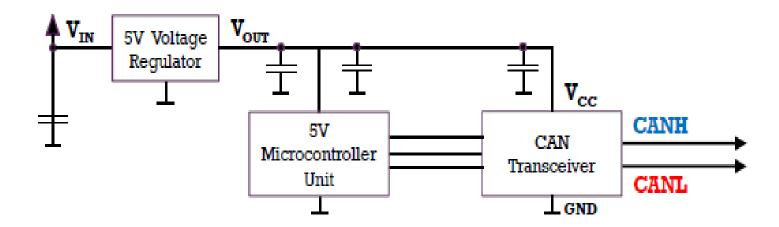
Figure 4: CAN typical application schematic.
