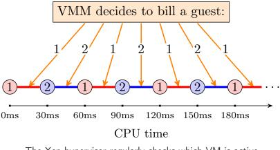
The Xen hypervisor regularly checks which VM is active to determine how much CPU time each VM uses
